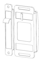
The distance between the two components must not exceed 15mm.
